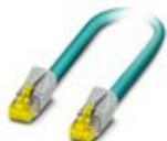
Patch cable, CAT6<sub>A</sub>, 4-pair, shielded, connection not crossed (line), assembled at both ends with RJ45/IP20 connectors, outer sheath material: PUR, length: 3.0 m
